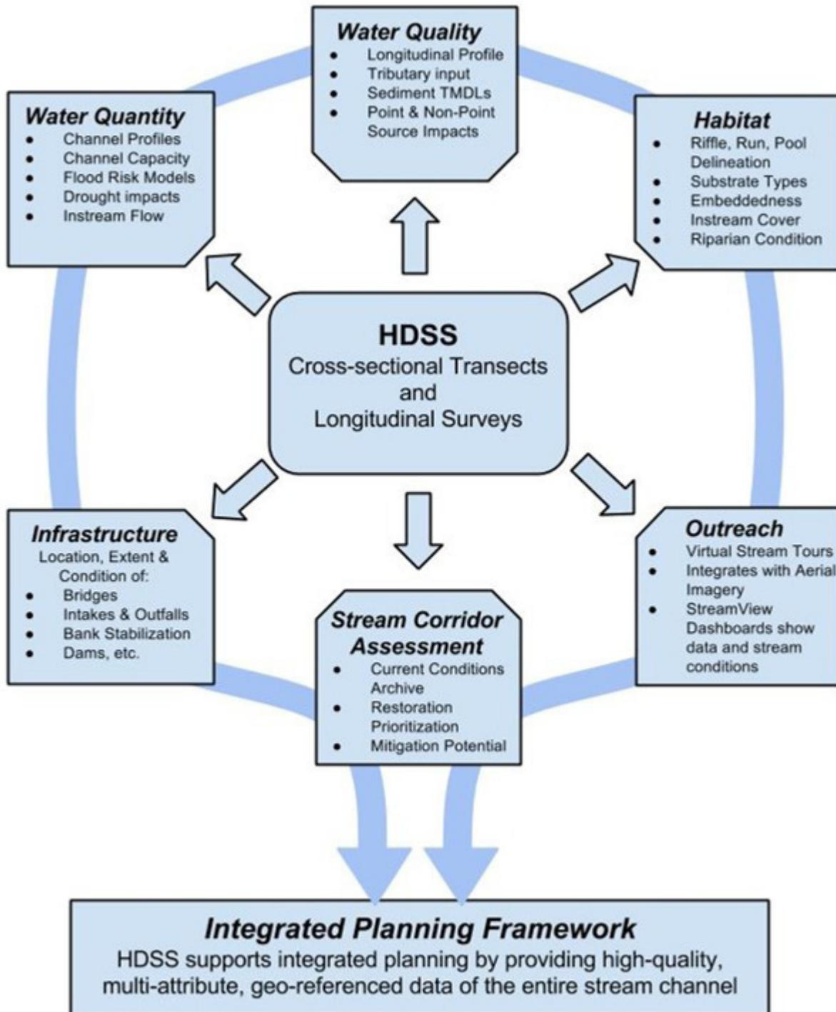
*HDSS allows for a single survey to gather information for numerous user groups for multiple applications. HDSS documents infrastructure for permits, precise bathymetry measurements for water quantity and quality modeling, and habitat parameters to prioritize mitigation work and protect and conserve aquatic resources.*
